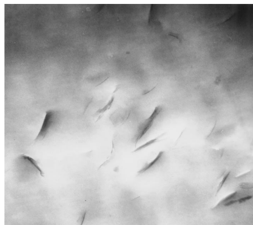
Figure 4 TEM micrographs of the ultrathin-section of C_{16}H_{33}(CH_3)_3N^+ -MMT/PI hybrid film containing 3.2 wt% MMT.
